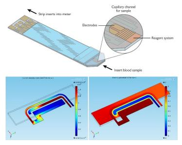
It is impossible to measure the potential drop across the electrodes or within the electrolyte in the measurement cell without physically disturbing the system. Modeling enabled the Roche team to isolate the chemical reactions from the electrical, mechanical, and temperature conditions so that they could analyze the voltage response.
