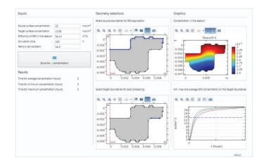
In one situation, to meet sterilization standards for classification of vials as novel containers, modeling ethylene oxide diffusion throughout the vials made it possible to adjust the required sterilization process without costly iterations.
