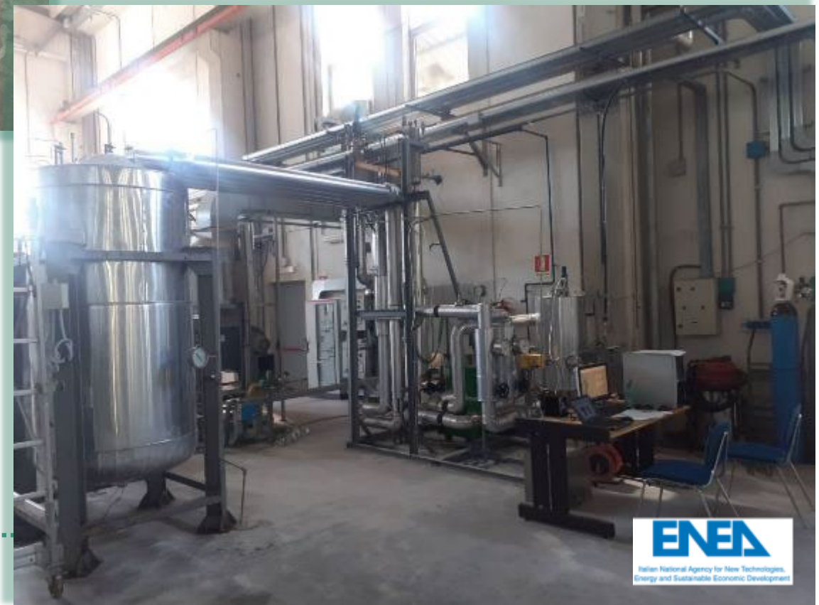
TES-SG prototype with oil loops
