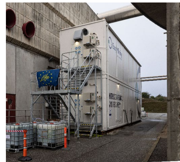
Photo: EasyMining Aqua2N process EU LIFE Re-Fertilizer project demonstration unit www.phosphorusplatform.eu/Scope145
