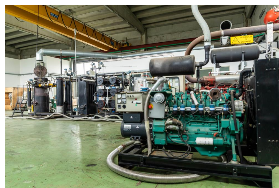
Internal combustion engine coupled with fixed bed downdraft gasifier for CHP
