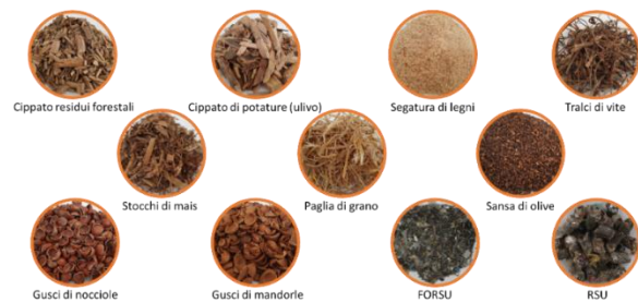
Figure 3. Feedstock specimens to be processed in the downdraft gasification reactor.
