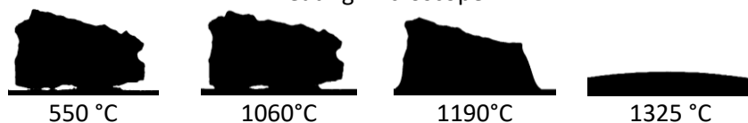
Figure 5. Ash agglomerates and equipment for characterizing their hardness and fusibility.
