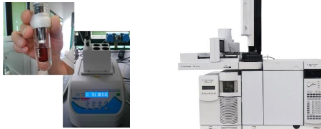
Figure 6. Sampling of condensation waste and analysis chromatographic systems (GCMS, HPLC)
