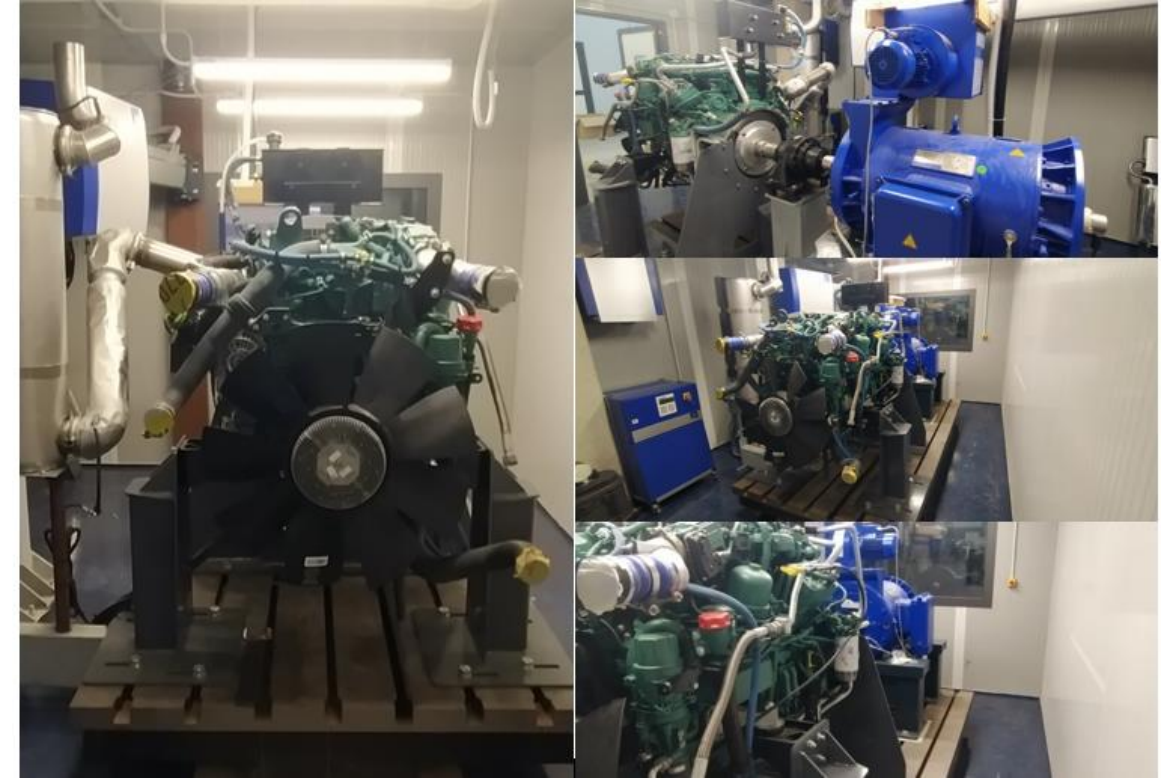
Diesel engine installed on a test bench for a complete performance characterization and for assessment of data acquired on-field
